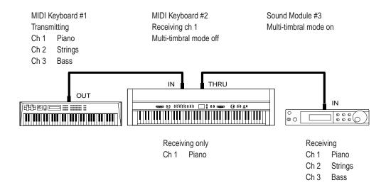
Instrument #2 recognizes only the piano part received from Instrument #1. Instrument #3 receives all the parts on the three channels being passed through Instrument #2 because Instrument #3's multi-timbral mode capability is activated.
